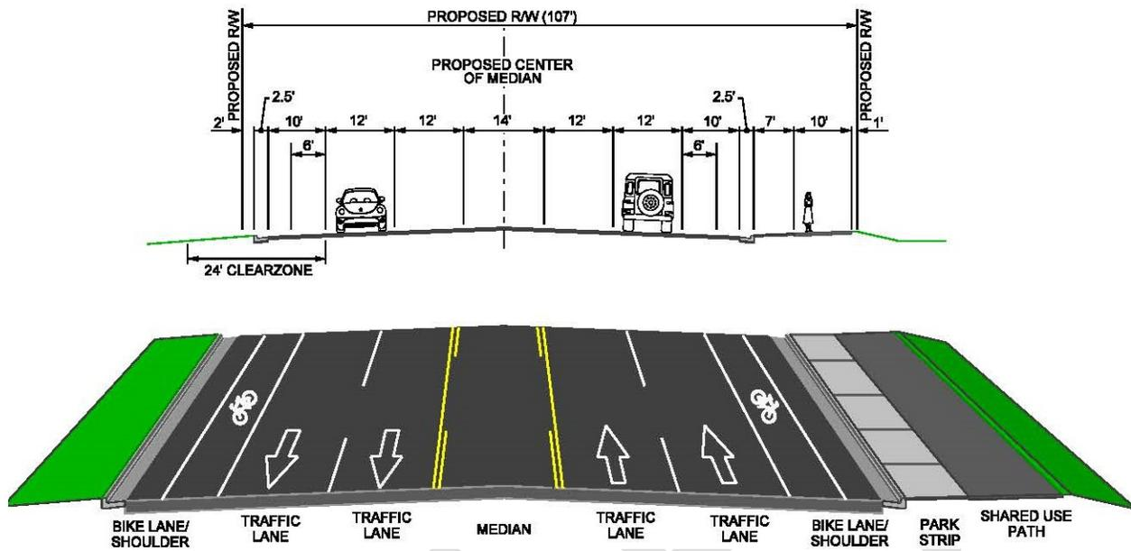
Figure 2-5. Multiple Roundabouts Alternative
