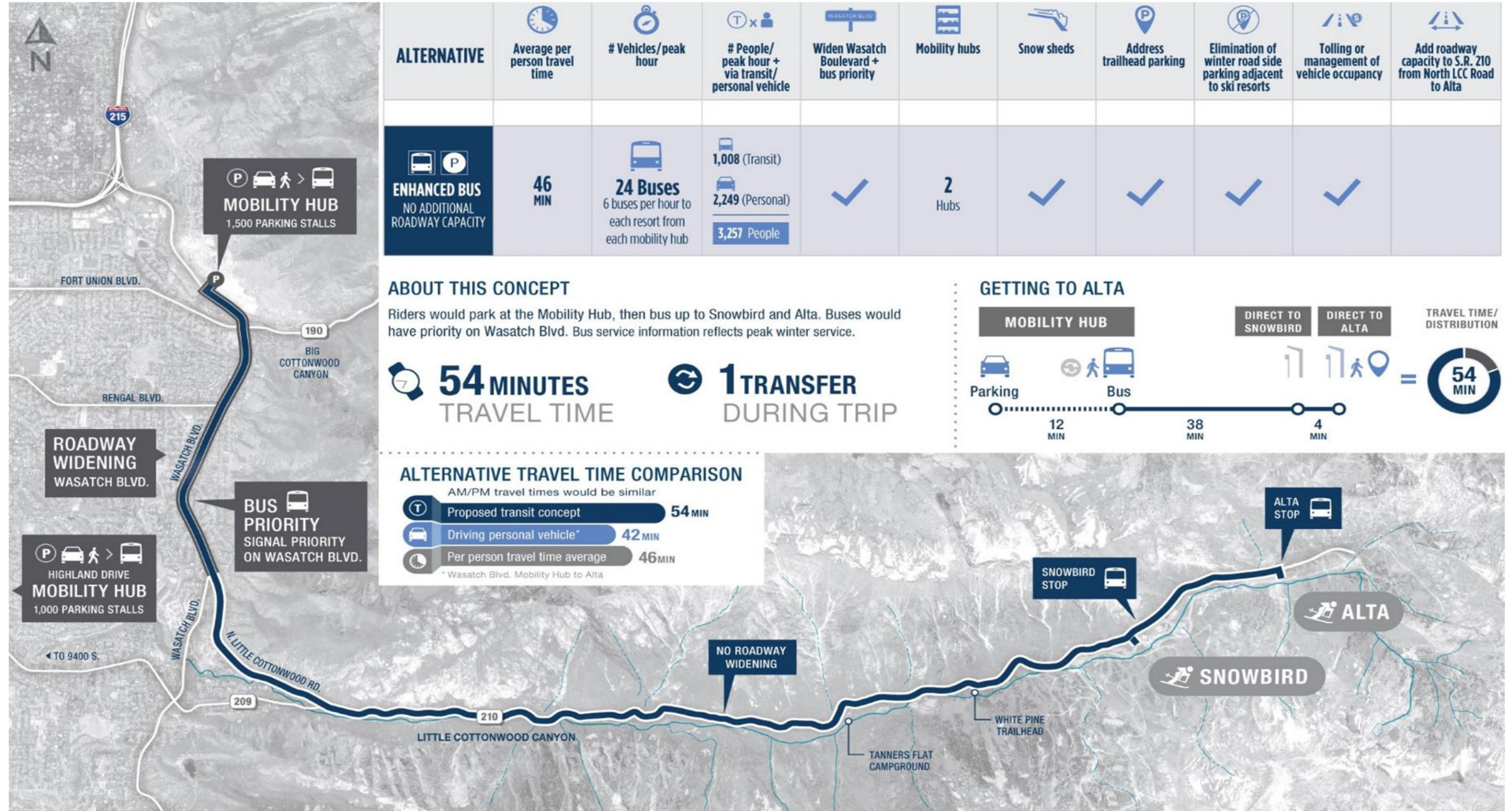
Figure S-4. Enhanced Bus Service in Peak-period Shoulder Lane Alternative
