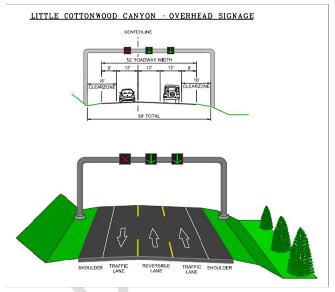
For S.R. 210, lane-control signals would indicate that two lanes are open to eastbound traffic and one lane is open to westbound traffic during the morning peak on peak traffic days. After the peak morning traffic passed, the signal for the center lane would shift to indicate that two lanes are open to westbound traffic and one lane is open to eastbound traffic.
