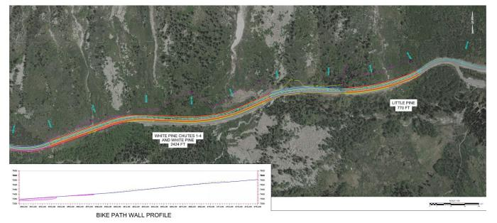
Moving the road and widening it toward the mountain side would also reduce the amount of fill or walls required on the downhill or stream side for the widened road and the bicycle lane that would be outside the sheds. The geotechnical composition and bedrock locations of the new roadway area were not evaluated.
